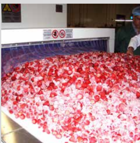
➤ Defrosting of IQF strawberries 1000 Kg/h throughput
