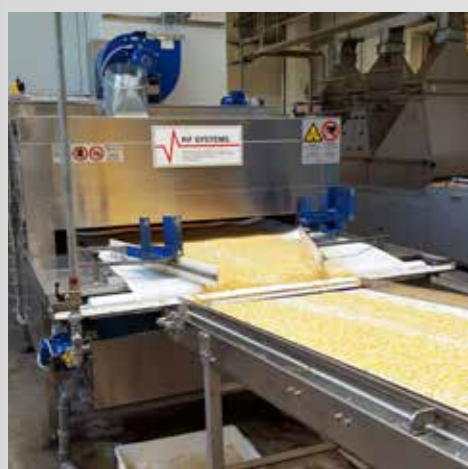
➤ Sanitization of corn 1000 Kg/h throughput
