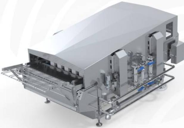
The cured sausage moisturizing unit for high performance is composed by a completely automatic water management system it allows to reuse the water by continuous filtering through a double filter. Automatic filling system by electrovalves, water level and temperature management.
